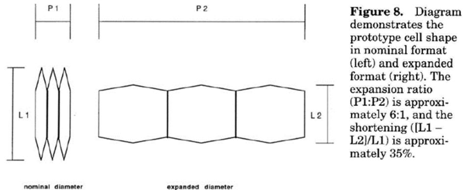
**Figure 8.** Diagram demonstrates the prototype cell shape in nominal format (left) and expanded format (right). The expansion ratio (P1:P2) is approximately 6:1, and the shortening ((L1 - L2)/L1) is approximately 35%.
